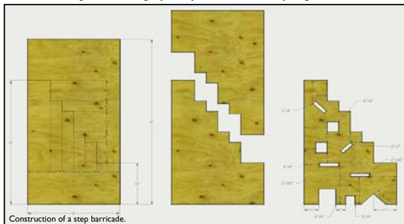
Construction of a step barricade.
